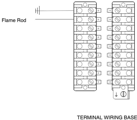
When wiring to the FLAME-MONITOR control wiring base, scanner terminal S2 must be grounded when using a flame rod. When using an infrared scanner (48PT2), ground S2 on all EB700's labeled "ENG CODE 00." All other ENG CODE models do not require that S2 be grounded. *Do not* ground S2 when using ultra violet scanners.
