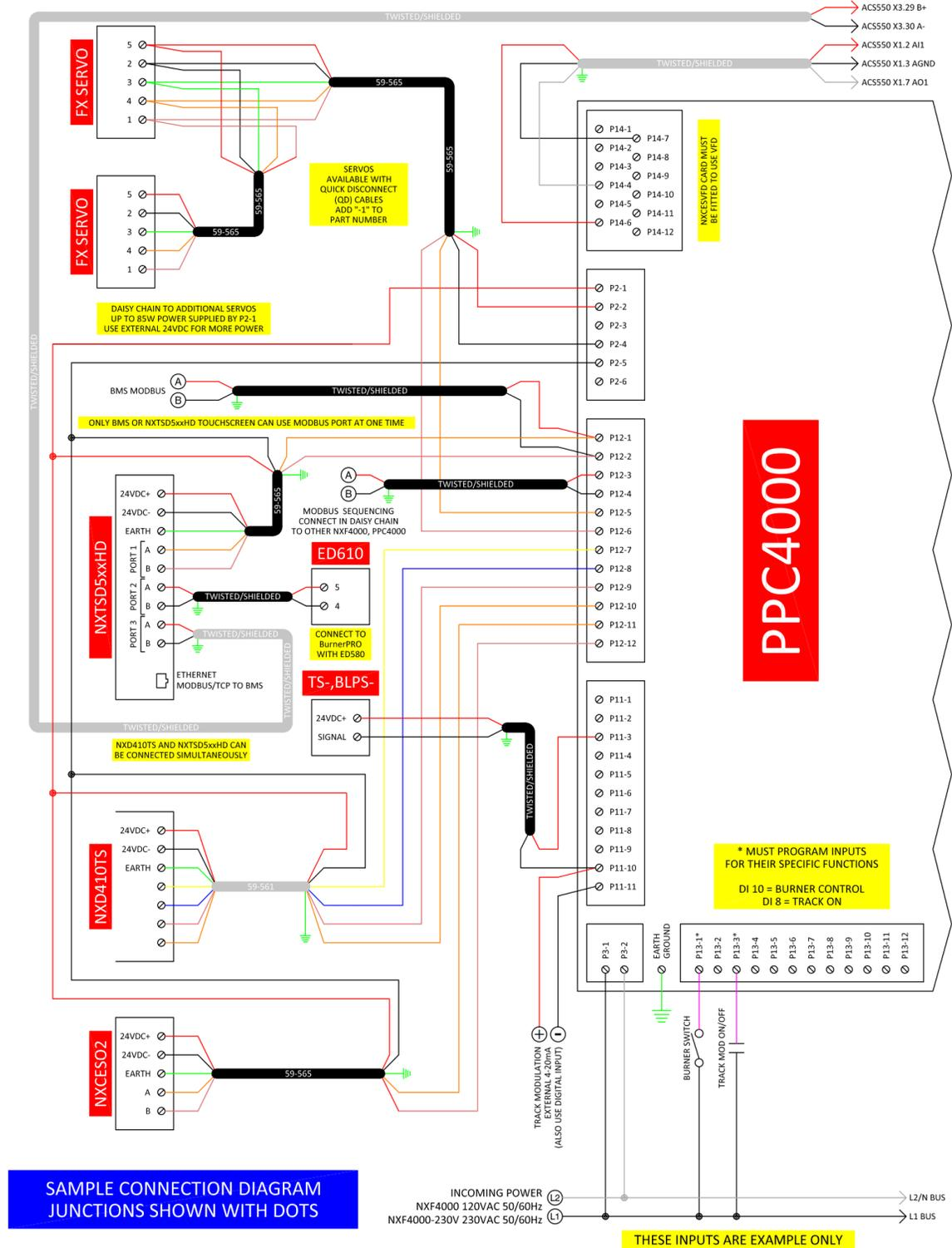
SAMPLE CONNECTION DIAGRAM JUNCTIONS SHOWN WITH DOTS
