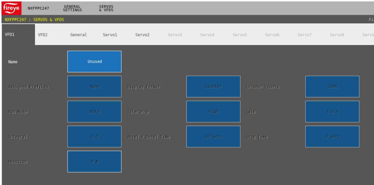
To enable the VFD for use, a name must be selected for the VFD. All the same names are available as with the servos and the same rules apply (at least one servo or VFD must be named AIR).
