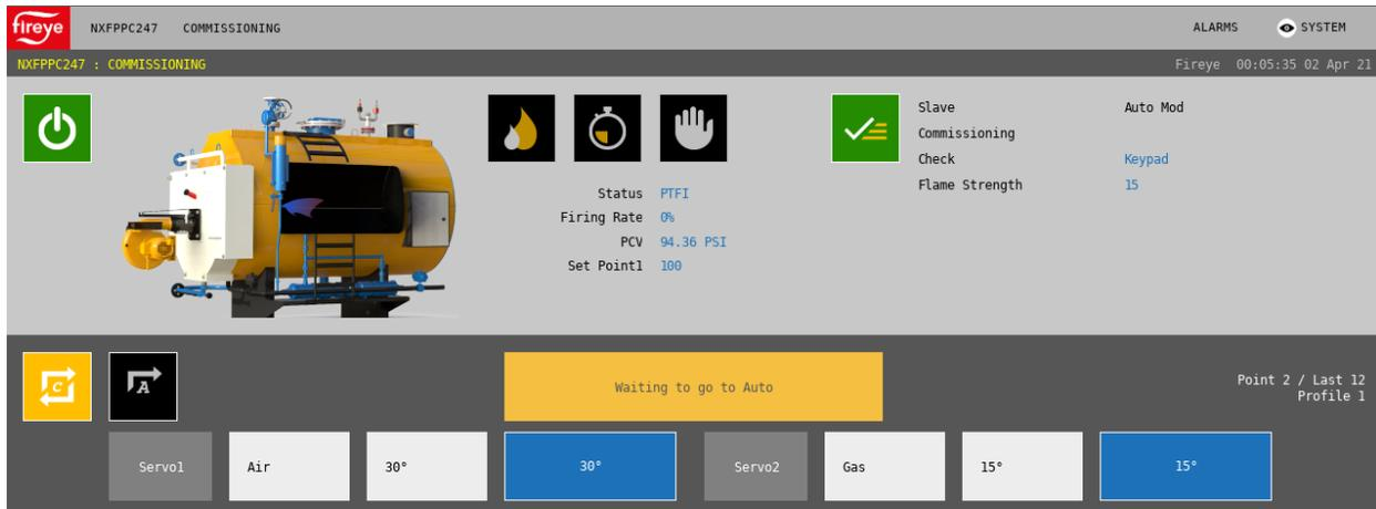
To confirm p02, exit check mode using the CHECK/RUN quick key and allow PTFI to complete. The NXF4000 will transition to MOVE TO LOW FIRE and allow p03 (first user defined point) to be commissioned. The NXTSD507HD and NXTSD512HD will both display a yellow banner MOVING TO POSITION P02 as the control purges.
