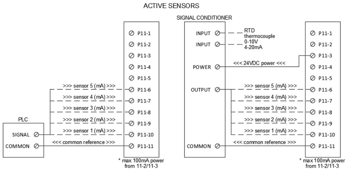
It is recommended that shielded cable is used to connect any remote mounted sensor. Only ground the shield on one side of the connection to prevent ground loops. It is not necessary to use shielded cable when wiring a signal conditioner to the NXF4000 or PPC4000 if it is in close proximity (same enclosure) but shielded cable should be used from the remote sensor to the signal conditioner.
