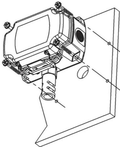
*FXIATS-140 temperature transmitter installation*
