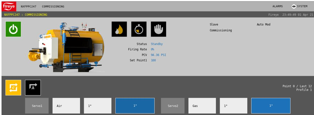
**NXF4000:** Once the burner on/off switch is set, the burner sequence will start and p01 can be commissioned.
