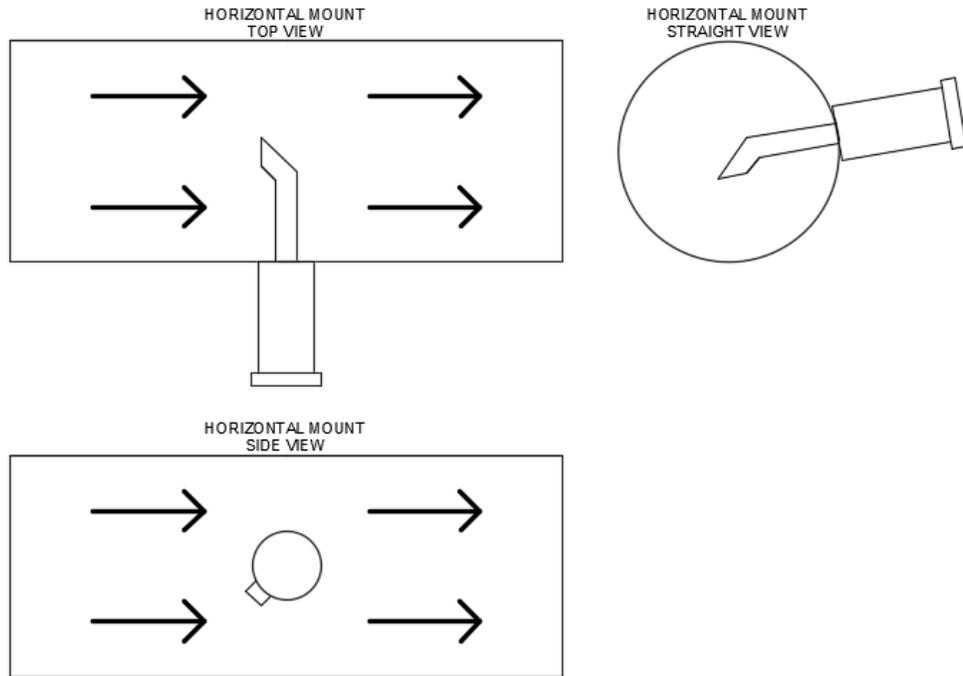
*Alternate mounting when stack is horizontal (acceptable)*
