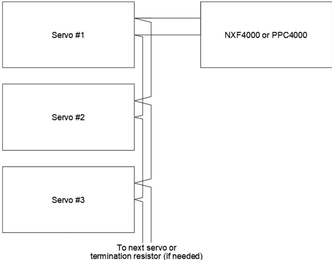
Never wire the servos in a star topology. This means to wire each servo directly to the Modbus terminals on the NXF4000 or PPC4000. Doing so will likely result in communication faults.
