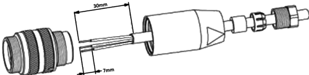
As shown above the cable strip length is specified at 30 mm (1.2 in) and each wire strip length is 7 mm (0.275 in).
