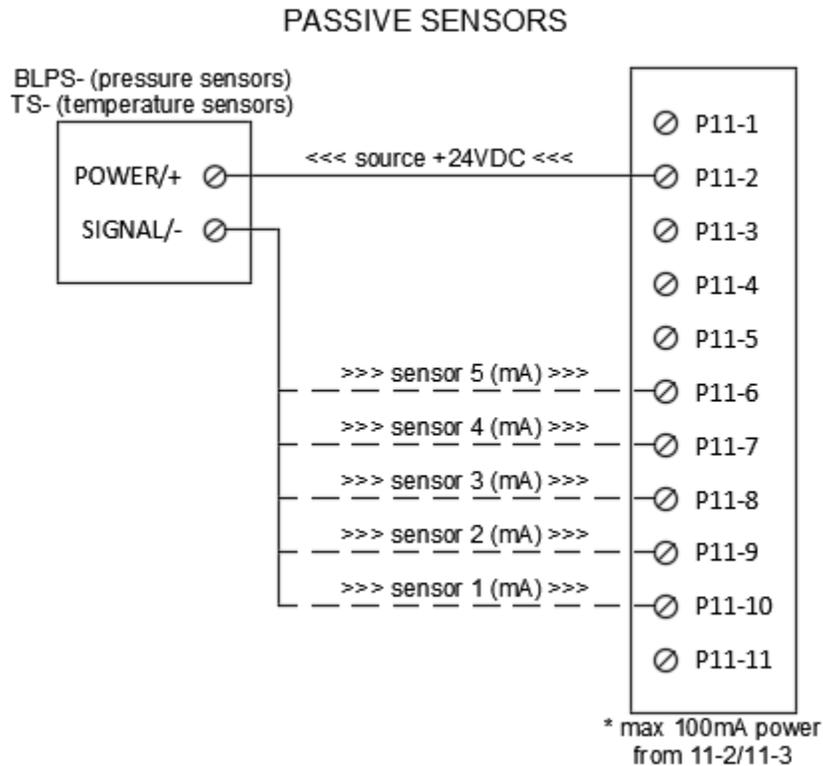
It is recommended that shielded cable is used to connect any sensor. Only ground the shield on one side of the connection to prevent ground loops.
