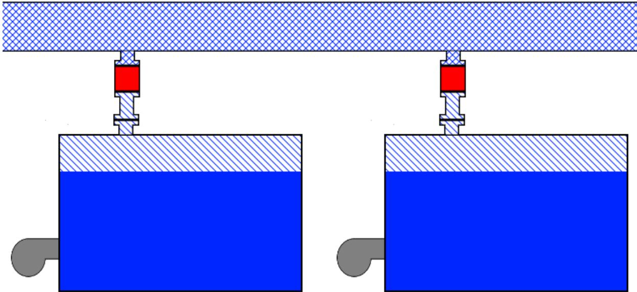
Boiler 1 is running and producing 6.89 Bar (100psi), which is going into the header. The non-return valve is keeping the steam out of boiler 2, which is not making any steam and is cold since it has been off for several days.
