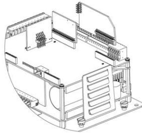
The NXCESVFD offers interfaces for up to two VFDs with either encoder feedback or with 4-20mA feedback from the VFD. The analog outputs from any unused channels can be used as user-assignable analog outputs.
