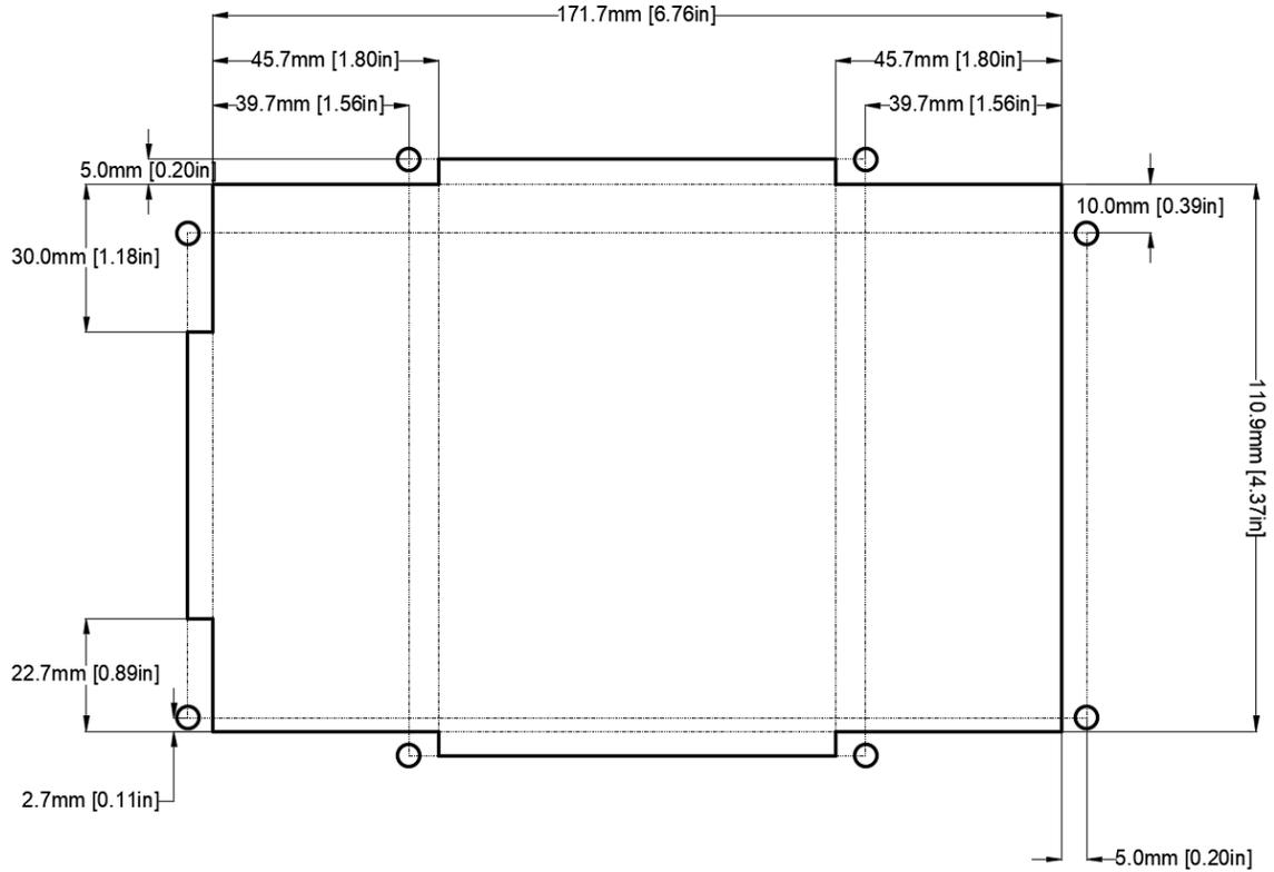
Holes are for M4x0.7 threaded posts with knurled-head thumb nuts (minimum clearance shown)
