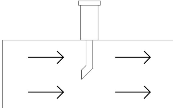
*Alternate mounting when stack is horizontal (preferred)*
