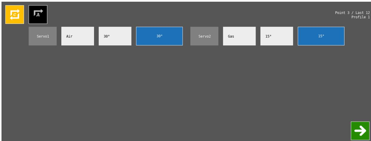
Since the gas regulator has been set already to make rate at the high fire position (see previous step), set the gas servo position based upon where the turndown can be verified, either by a fuel flow meter or by clocking the meter. It is important to check that the expected turndown is being delivered.
