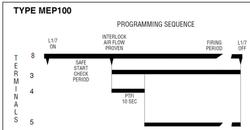
Terminal #5 is energized 3 seconds after flame is detected.
