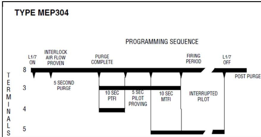
0 Second post purge on operating control open. 15 Second post purge on flame fail.
