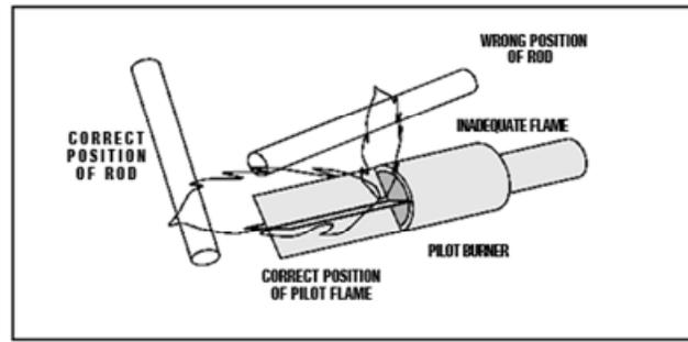
4. If the flame is nonluminous (air and gas mixed before burning), the electrode tip should extend at least 1/2" into the flame, but not more than halfway through.
