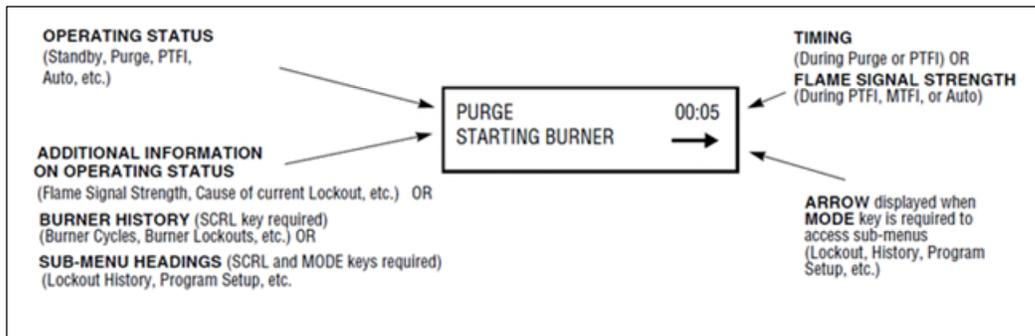
At any time the MicroM is powered, the SCRL key is used to scroll through and display the total number burner hours, burner cycles, burner lockouts and system hours on the bottom line of the ED510 display. The top line will continue to show the current run mode of the control (e.g. PURGE, AUTO, etc.) Following the historical information, the SCRL key will display three (3) sub-menus providing the following information and/or functions:
