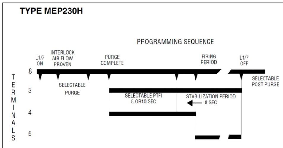
Pilot Stabilization timing begins as soon as flame is proven.
