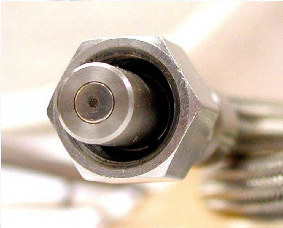
The cable ends have stainless steel fittings with compression fitting nuts and ferrules to mate and seal with the FSA and the electronics enclosure (ends are fully interchangeable).
