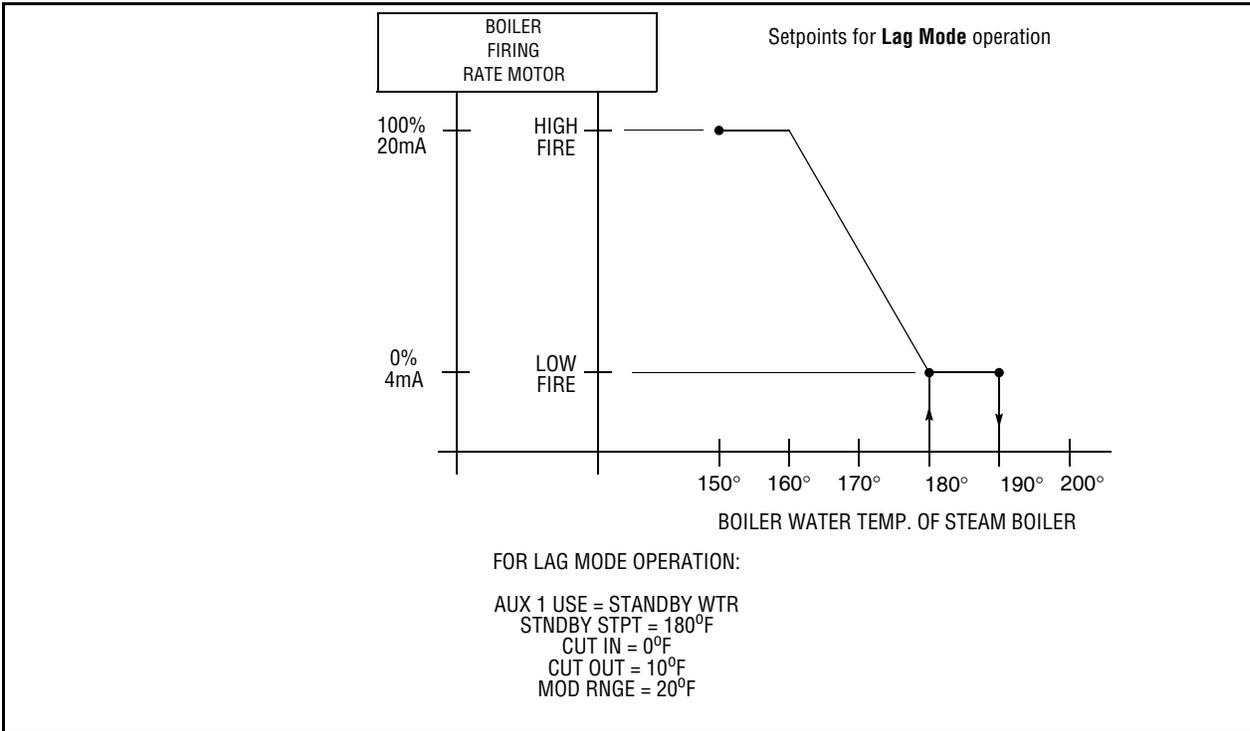
**STANDBY THERMAL SHOCK PROTECTION MODE:**
