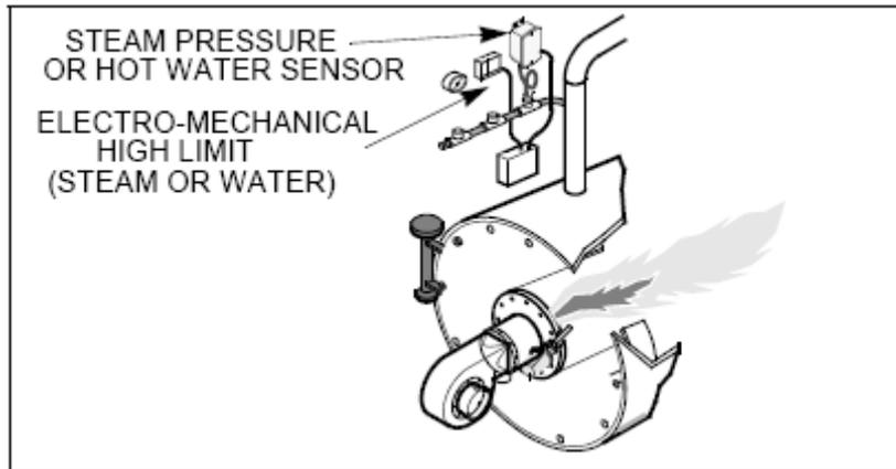
7. Although the unit can withstand substantial vibration without damage or significant output effects, it is good practice to mount the pressure sensor where there is minimum vibration.
