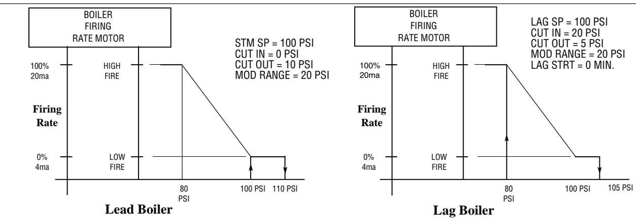
**EXAMPLE 2:** The Lead Boiler attempts to control the steam pressure at 100 PSI. As demand increases and steam pressure drops, the Lag Boiler cuts in at 80PSI and immediately drive to the high fire position. As steam pressure increases, both boilers decrease their firing rate. At 105 PSI, the Lag Boiler cuts out. It won't cut in until steam pressure again drops to 80 PSI. The Lead Boiler cuts out at 110 PSI and cuts in at its steam pressure set point (100 PSI).
