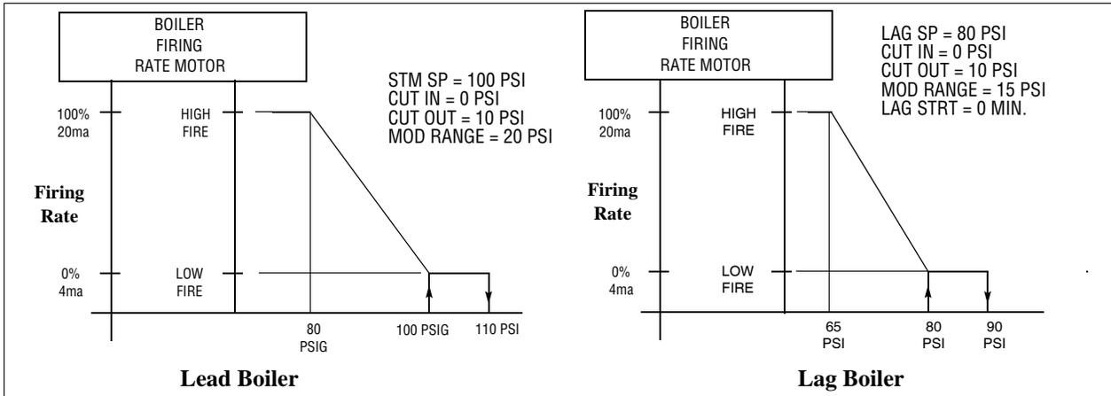
**EXAMPLE 1:** The Lead Boiler attempts to control the steam pressure at 100 PSI. As demand increases and steam pressure drops, the Lag Boiler cuts in at 80PSI at the low fire position. The Lag Boiler modulates from low to high fire between 80 PSI (low fire) and 65 PSI (high fire). As steam pressure rises, the Lag Boiler cuts out at 90 PSI. At 90 PSI, the Lead Boiler is at mid range of its firing rate.
