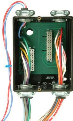
***NOTE:** The Phoenix QDWR models with electrical quick-disconnect have replaced the original WR models equipped with ten feet of captive cable. The QDWR models (with 59-546-X cables) are also suitable for use in Class I Division 2 hazardous areas, thereby eliminating the need for the "EXWR" models.*
