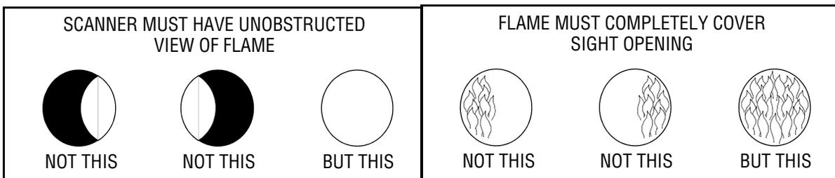
5. Smoke or unburned combustion gases absorb ultra-violet energy. On installations with negative pressure combustion chambers, a small hole drilled in the UV1A, UV2 sight pipe will assist in keeping the pipe clean and free from smoke. Provide clean air to pressurize the sight pipe, if necessary for positive pressure furnaces.
