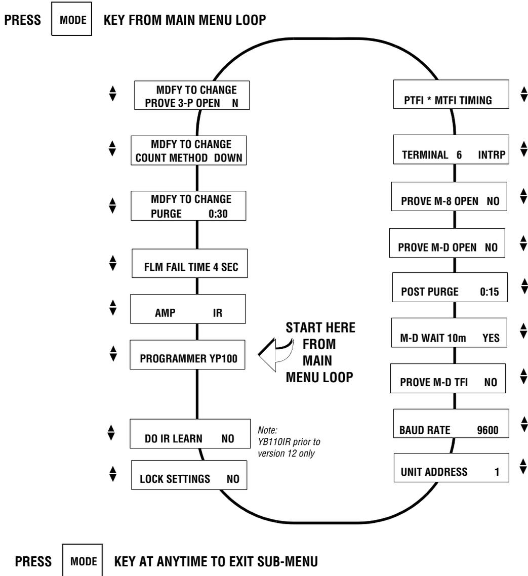
**Table 15: MODIFIABLE PARAMETERS LOCATED IN PROGRAM SETUP MENU**
