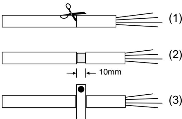
(1) The cable should be prepared by cutting around the outer insulation, taking care not to damage the screen (1).
