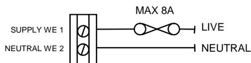
The LIVE and NEUTRAL supplies must be connected using multi-strand single core PVC insulated 16/0.2mm wire. The live connection should be fused with a **maximum rating** as shown. **If a fuse greater than 4A is fitted, each relay (pump, fan and vent) output supplied via this terminal MUST be separately fused at 4A maximum, to protect the relay contacts from 'welding'.**
