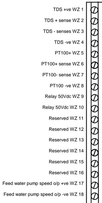
The cabling for all of these terminals MUST be overall 'braid' screened, PVC insulated, 7/0.2mm, 2-core. As this cable may lay adjacent to, and/or in the same conduit as Line voltage wiring, the cable voltage rating must exceed the maximum voltage carried by any other cable connected to the controller or run in the same conduit.
