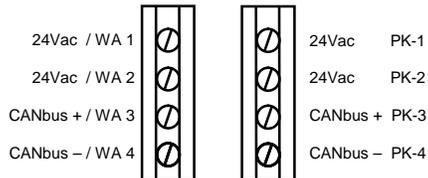
CANbus allows several options for connecting the devices together, based on the physical position of each device relative to the main controller and the current required by each device. The recommended cable is overall 'braid' screened, PVC insulated, 4-core, 7/0.2mm wire, which has a maximum current carrying capability at 60°C (140°F) of 600mA. This
