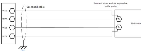
Acceptable wiring scheme for 2 terminal TDS probe.
