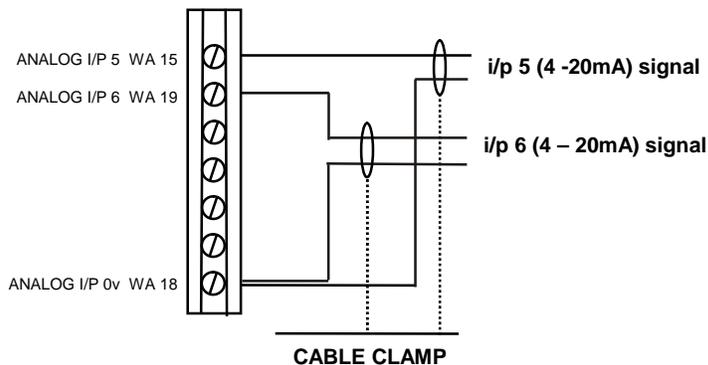
Connect the cable 'braid' screen to the controller with the use of the screen termination clamp. Make all connections at the sensor/transmitter first.
