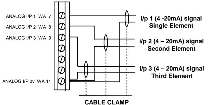
The pressure sensor cabling **MUST** be overall 'braid' screened PVC insulated 7/0.2mm (number of cores as required by the relevant sensor). As this cable may lay adjacent to, and/or in the same conduit as Line voltage wiring, the cable voltage rating must exceed the maximum voltage carried by any other cable connected to the controller or run in the same conduit.
