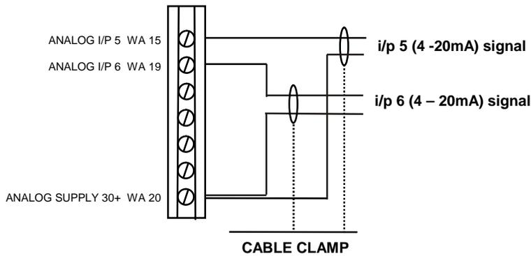
Connect the cable 'braid' screen to the controller with the use of the screen termination clamp. Make all connections at the sensor/transmitter first.
