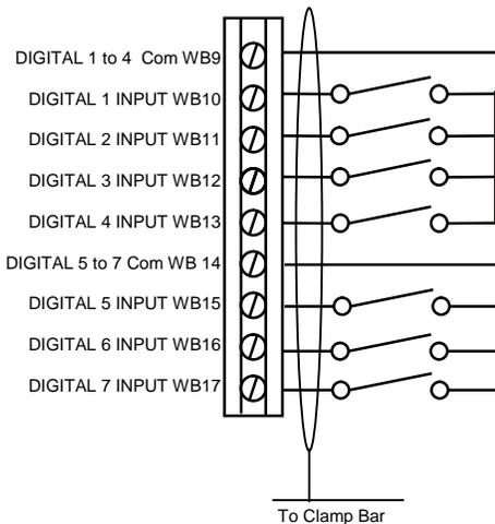
These Low Voltage digital inputs can be used for safety related functions and their function is programmed by option parameters 68.1 to 68.7 inclusive.
