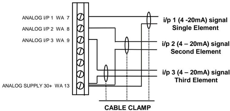
The pressure sensor cabling **MUST** be overall 'braid' screened PVC insulated 7/0.2mm (number of cores as required by the relevant sensor). As this cable may lay adjacent to, and/or in the same conduit as Line voltage wiring, the cable voltage rating must exceed the maximum voltage carried by any other cable connected to the controller or run in the same conduit.
