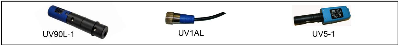
**CAUTION: The UV90L-1, UV1AL, and UV5-1 flame scanners are non-self checking UV sensors. Use these only on burners that cycle often (e.g.: a minimum of once every 24 hours) in order for the external safety checking circuit to be exercised.**
