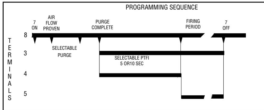
Selectable Recycle/Non-Recycle operation on loss of flame after Terminal 5 energized. Recycle on loss of air flow after flame proven.
