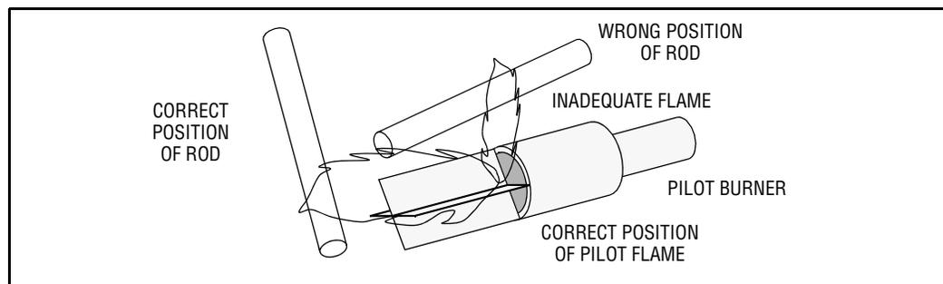
5. If the flame is partly luminous, the electrode tip should extend only to the edge of the flame. It is not necessary to maintain absolutely uninterrupted contact with the flame.
