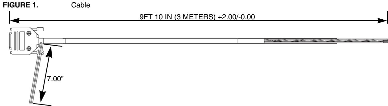
The DA15-FM connector plugs into the PLC port located on the backside of the NXD410 as shown in Figure 2. The cable distance from the PPC4000 to the NXD410 is limited to 10 feet (3 meters) wire run.
