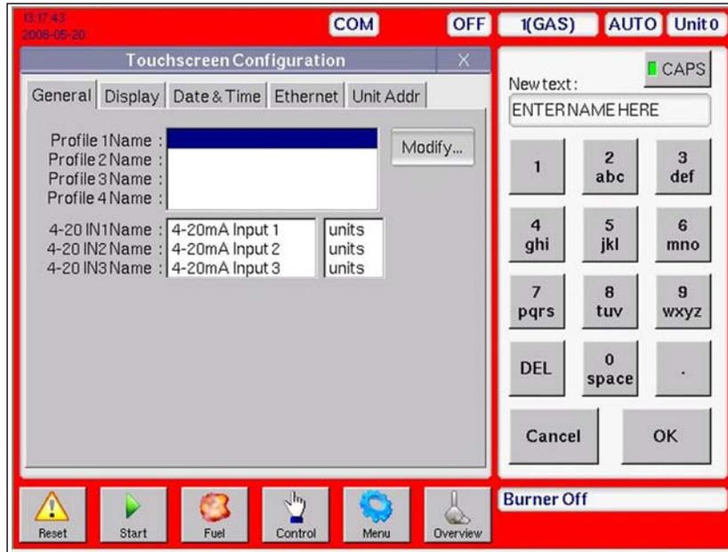
Highlight the profile for which a name is to be entered or modified and press the Modify button. This will cause a window to appear allowing the required name to be entered using the button pad.
