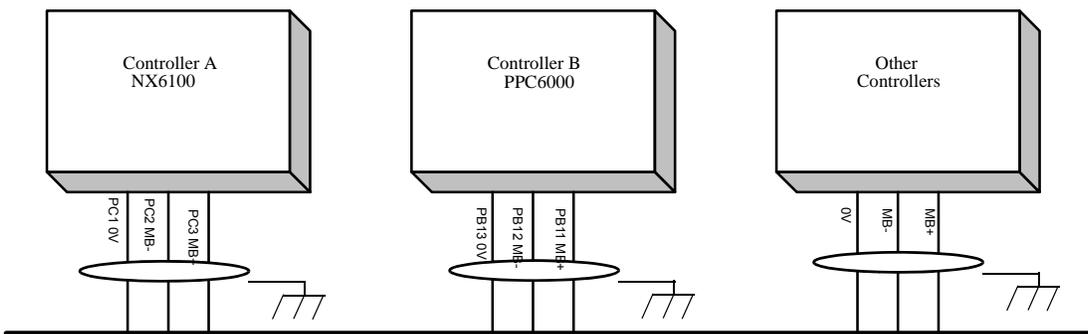
Figure 1: MODBUS Connections
