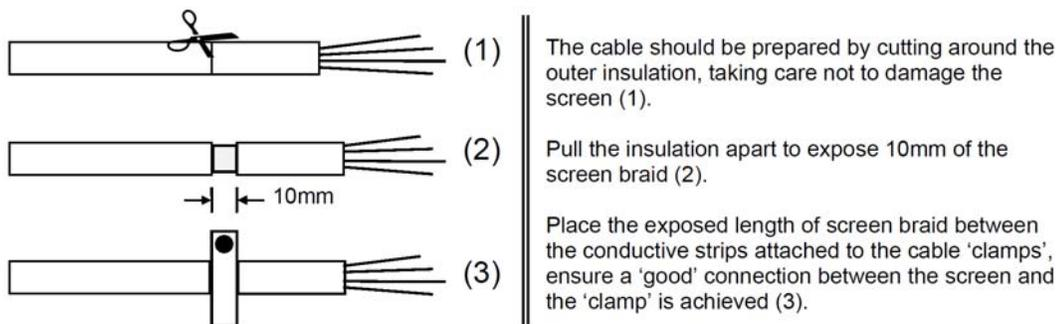
**NOTE: The 'clamps' are not intended to provide strain relief for the cables.**
