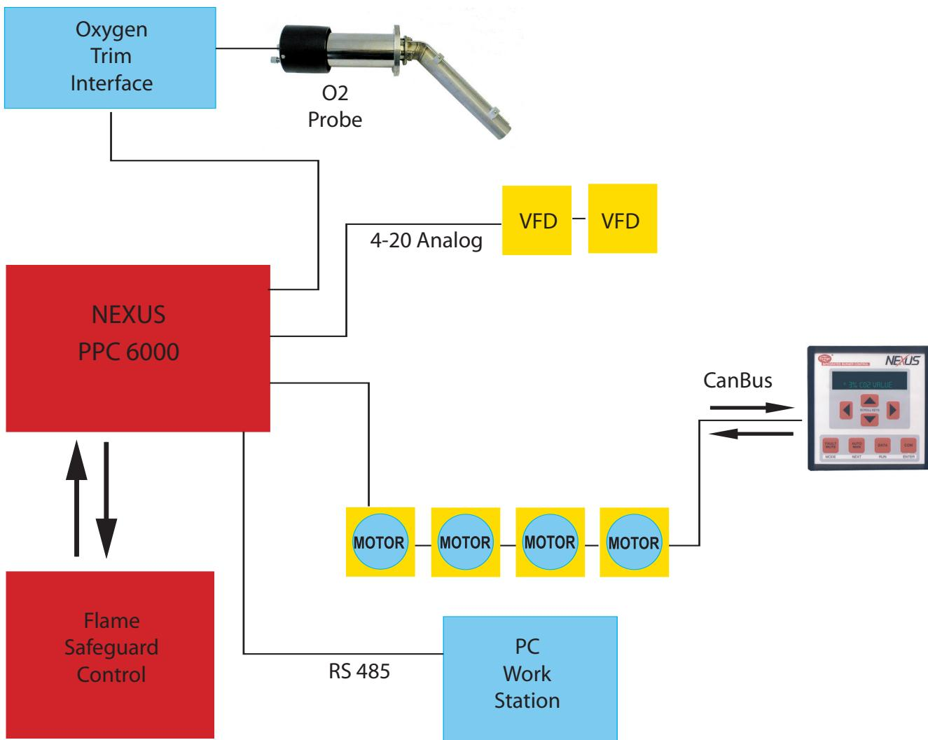
Variable speed interfaces are available to control, via inverters, the burner fan motor as well as FGR fans. Controlling the fuel/air ratio by adjustment of fan speed saves electrical energy and reduces noise. When the motor speed is halved an 80% electrical energy saving is achieved. Up to four variable speed interfaces can be added to a single PPC 6000. Another option of the PPC6000 is Oxygen trim control.
