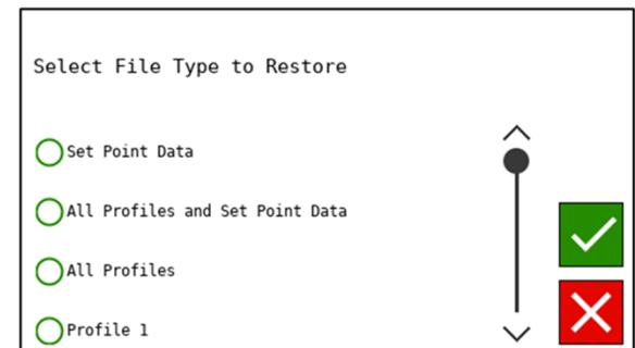
Once an option is chosen all available backup files are shown so the one to restore can be selected. If the backup file is invalid (corrupted or from an incompatible firmware or model such as the PPC4000), this will be indicated. Note that restoring can only be done when the control is in the standby state or the message will read NOT IN STANDBY.
