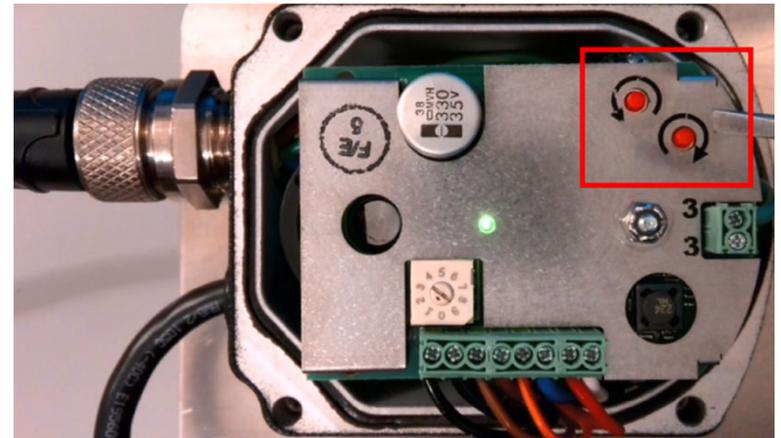
**For the exercise, first power up the unit. Then use the manual movement buttons to make sure each servo will go from 1° to 100° to simulate testing actual movement. Leave the servo at what will be the fully closed position (1°).**
