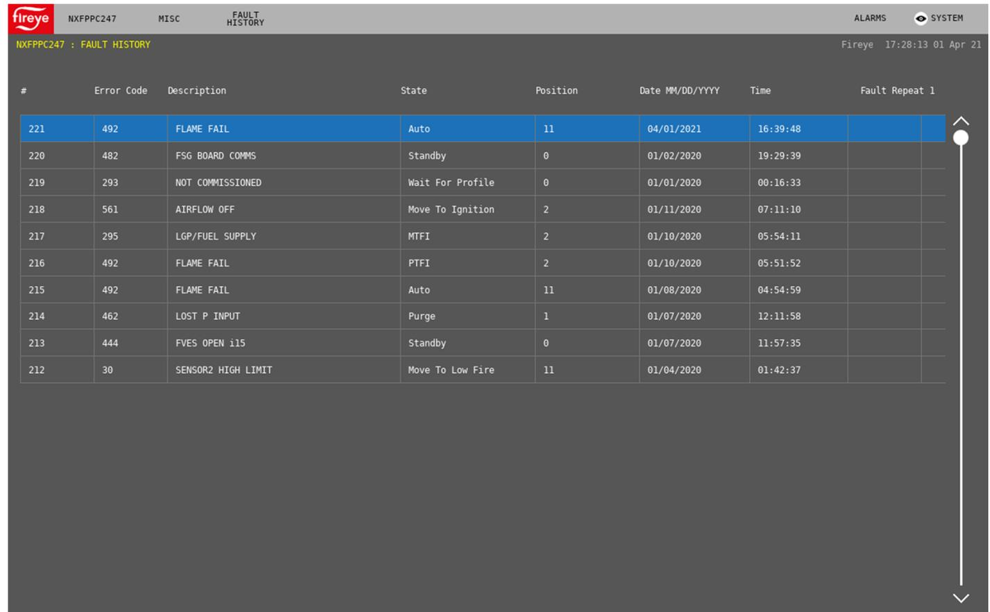
The screenshot shows the Fireye control interface for unit NXFPPC247. The 'FAULT HISTORY' tab is selected, displaying a table of error events. The table columns are: #, Error Code, Description, State, Position, Date MM/DD/YYYY, Time, and Fault Repeat 1. The table contains 10 rows of data, with the most recent entry (221) highlighted in blue.
