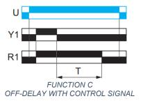
closed for duration T, which is typically set using dials or DIP switches. For this application the duration should only be set to one second. If power is removed from U, R1 will open immediately.
