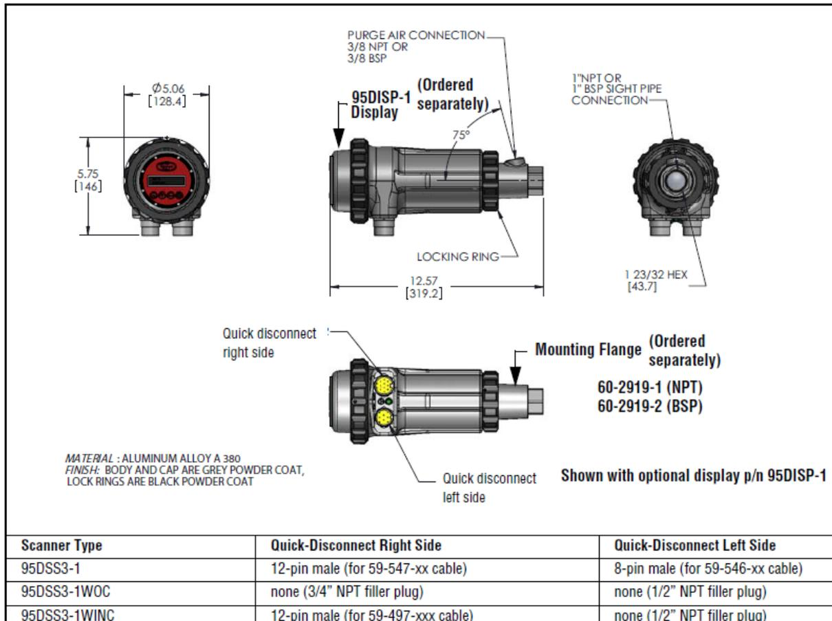
**FIGURE 2. TYPE 95DSS3-1CEX, -1WICEX, -1CEX-ND SCANNERS, STANDARD FLAME-PROOF HAZARDOUS AREA HOUSING**
