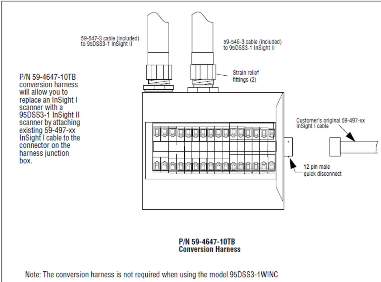
**FIGURE 20. WIRING DIAGRAM FOR P/N 59-4647-10TB CONVERSION HARNESS**
