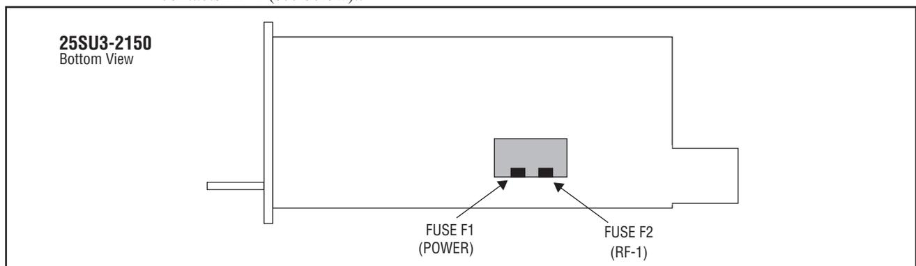
*Note:* Fuse F2 is not replaceable. If fuse F2 needs replacing, the amplifier **MUST** be sent back to manufacturer for replacement.
