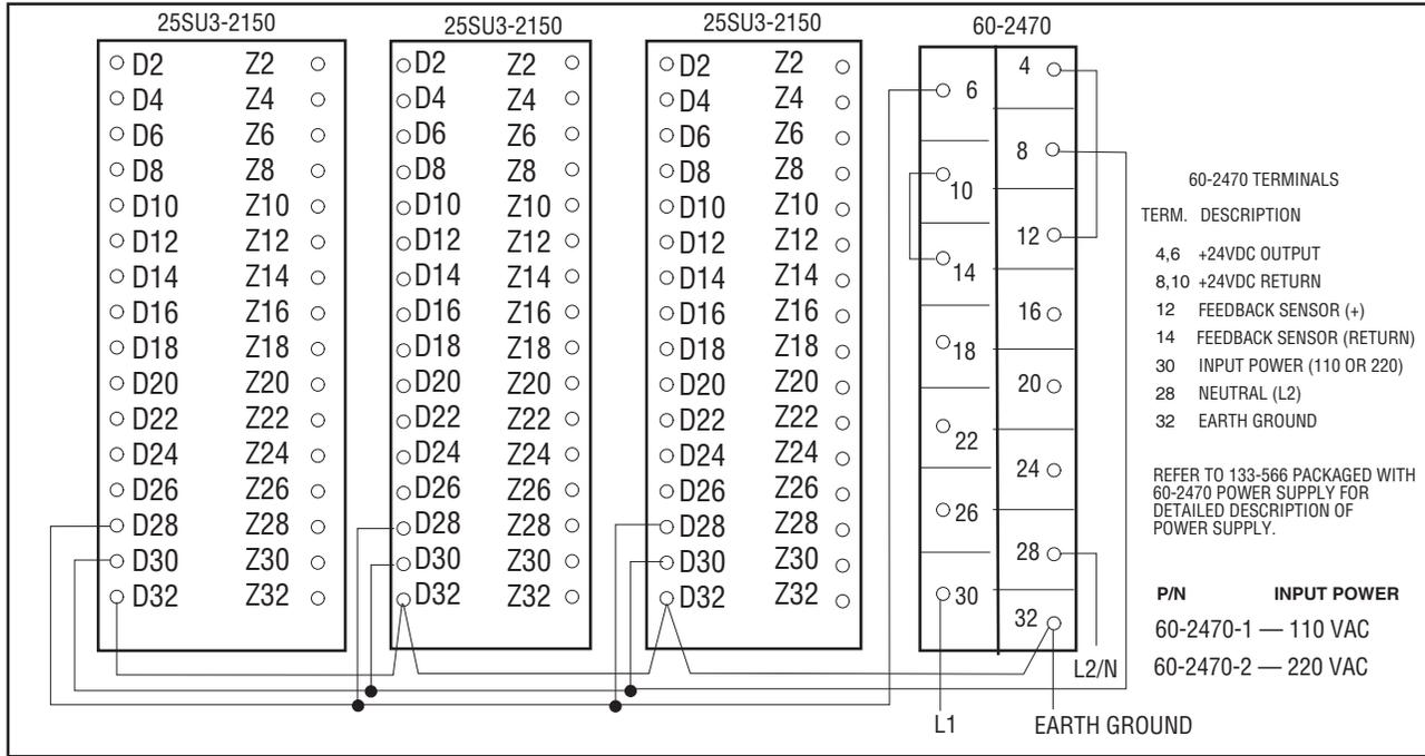
**FIGURE 9. 25SU3-2150 SCANNER WIRING DIAGRAM: (25SU3-2150 AMPLIFIER, 45RM4\*\* DC SCANNER WIRING COMBINATIONS<sup>1, 2</sup>)**
