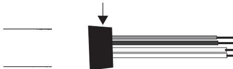
5. SECURE BRAIDED SHIELD AND CABLE JACKET TO BUS BAR. Use two metal clamps, flat washers and extended nuts (provided). (Scanner cables may enter bus bar from either top or bottom and use any two studs for each cable).
