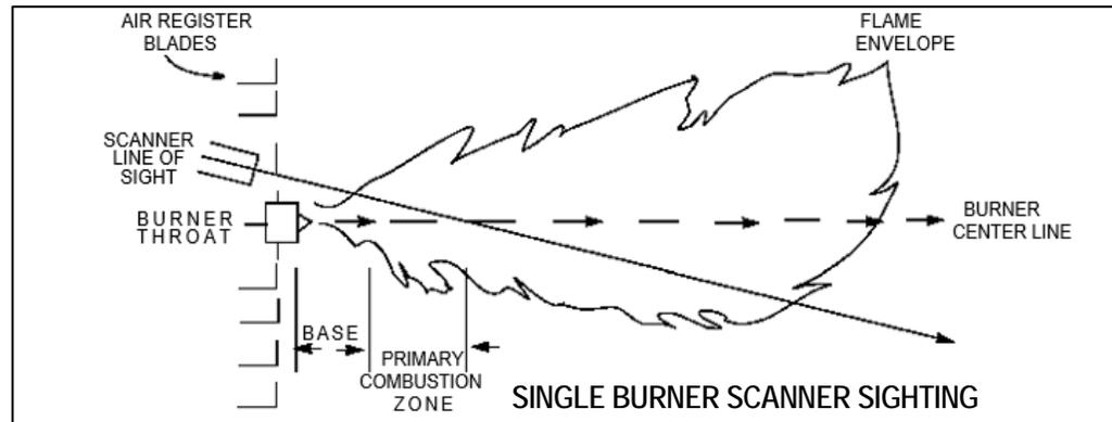
4. AN ACCEPTABLE SCANNER LOCATION MUST ENSURE THE FOLLOWING: — Reliable pilot flame detection.
