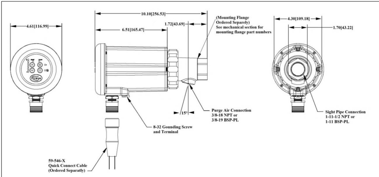
**FIGURE 2. PHOENIX SCANNER in ATEX HAZARDOUS AREA HOUSING (mounting flange kit ordered separately)**
