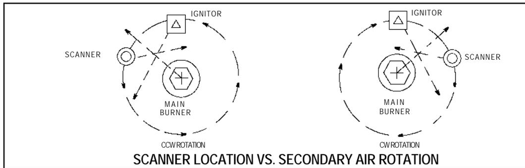
5. If combustion air enters the furnace with a rotational movement of sufficient velocity to deflect pilot flame in direction of rotation, position the scanner 0 to 30 degrees downstream of the pilot burner and close to the periphery of the throat where the ultraviolet radiation is at a maximum. (See Figures 3 and 4).
