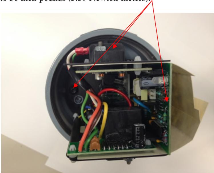
9. Reconnect the scanner cable wires to the two terminal strips on the electronics assembly.
